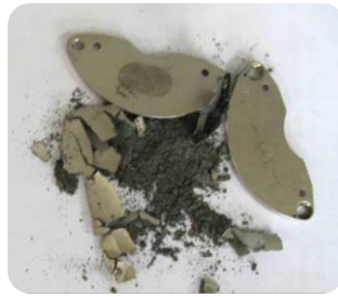
HPMS process demagnetises the rare earth magnet, producing NdFeB powder
